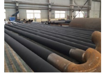
HiE-Coat™ 840-M coats gas-fired heating tubes.
