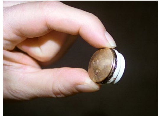
Aremco-Bond™ 570 bonds ceramic to copper nozzle.
