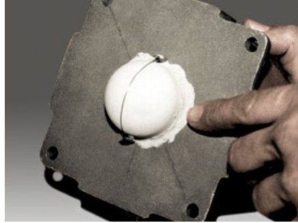
Cerabond™ 571 coats oxygen sensor.
