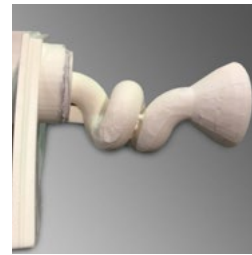
Ceramabond™ 503 coats spiral cantilevered sensor.
