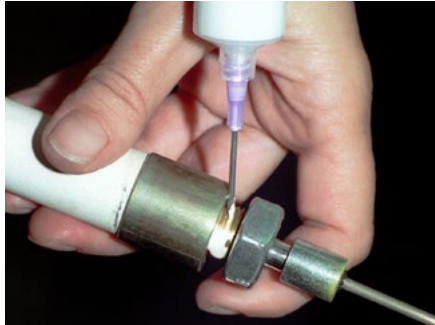
Cerabond™ 671 used as a high temp threadlocker.
