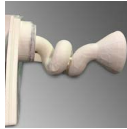
Ceramabond™ 503 coats spiral cantilevered sensor.
