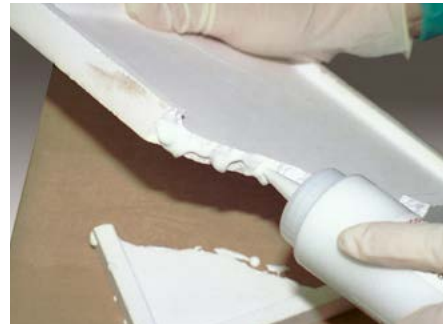
Cerabond™ 503 repairs furnace saggar plate.
