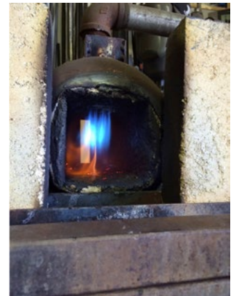
HiE-Coat™ 840-CX applied to a gas-fired forge.
