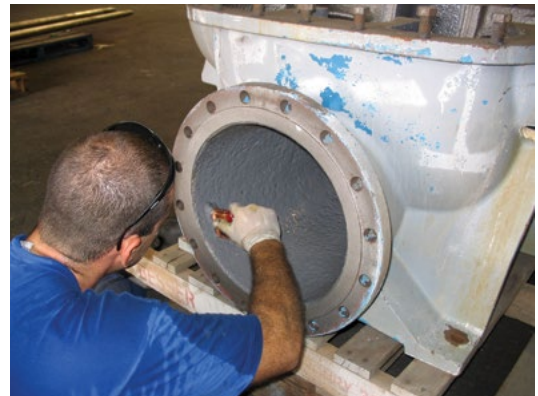
Corr-Paint™ CP2060 coats pump housing.
