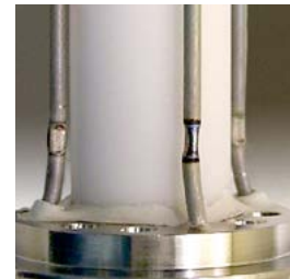
Ultra-Temp™ 516 seals heater assembly.
