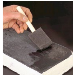
HiE-Coat™ 840-C coats ceramic fiberboard infrared heater.
