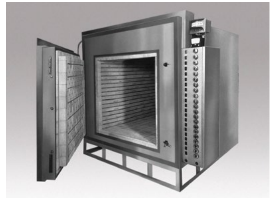
The Econo-Heat™ furnace shown is a custom unit designed for an aerospace manufacturer for use in heat treating. This furnace has a work area of 42" x 42" x 65", and a unique temperature control system consisting of 21 elements each with its own infinite control switch to permit uniform heating of complex shapes.
