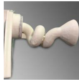
Ceramabond™ 503 coats spiral cantilevered sensor.
