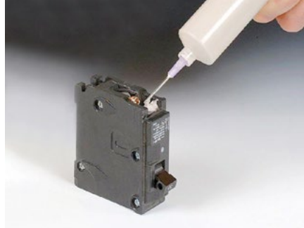
Ceramacoat™ 512-N insulates circuit breaker terminal.
