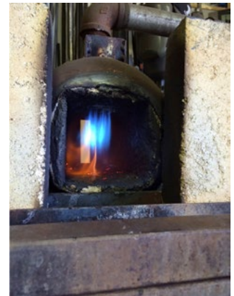
HiE-Coat™ 840-CX applied to a gas-fired forge.
