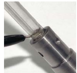
Aremco-Bond™ 631 bonds sapphire tube to stainless steel.
