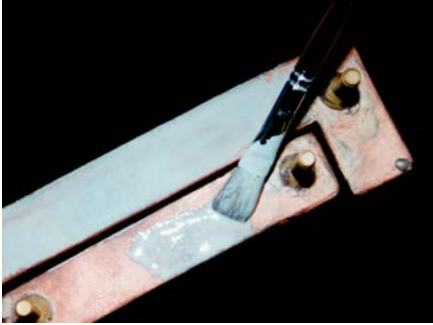
Cerabond™ 571 coats copper induction heater.
