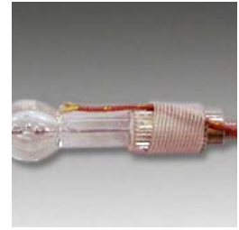
Ceramabond™ 503 coats heater used to 1700 °C.
