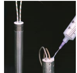
Ceramacast™ 586 pots ignitor and cartridge heater.
