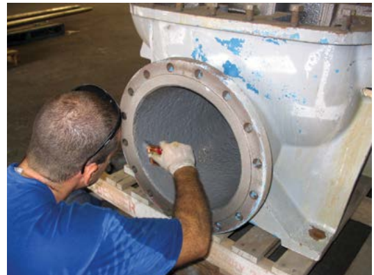
Corr-Paint™ CP2060 coats pump housing.
