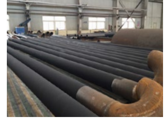
HiE-Coat™ 840-M coats gas-fired heating tubes.
