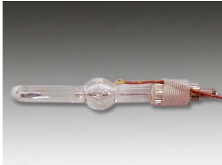
Ultra-Temp™ 516 bonds thermocouple to quartz tube.
