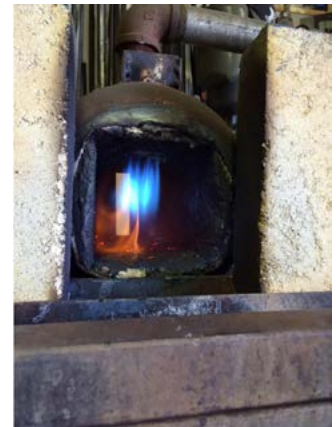
HiE-Coat™ 840-CX applied to a gas-fired forge.
