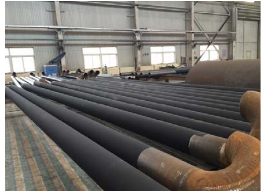
HiE-Coat™ 840-M coats gas-fired heating tubes.
