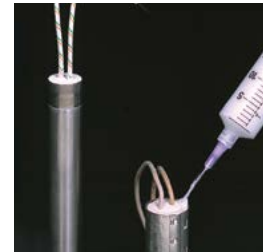
Ceramacast™ 586 pots ignitor and cartridge heater.
