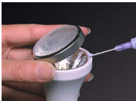
Cerabond™ 835-M bonds cover to halogen lamp.
