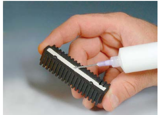
Ceramacast™ 586 pots high power resistor.
